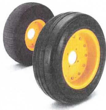
All Heavy-Duty Rotary Cutters are available with the durable laminate tire. The RC10R and RC14R pull-type models come with severe-duty ag tires for improved flotation on soft ground and smoother long-distance travel.
