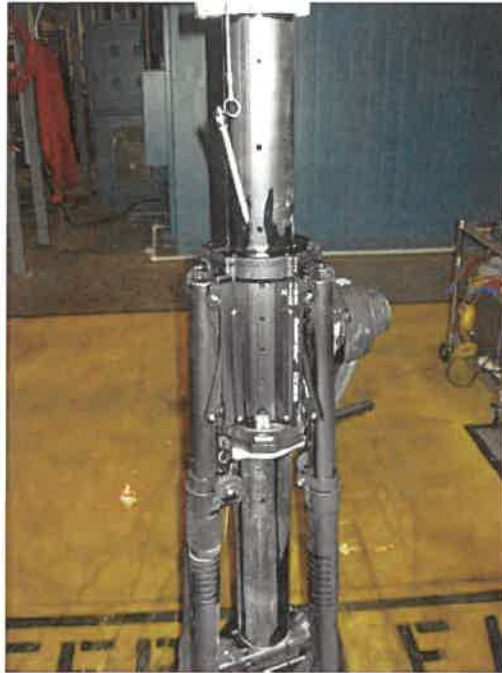
SALT FOG POST TEST – AFTER 48 HOUR DRYING PERIOD/CLEANING
